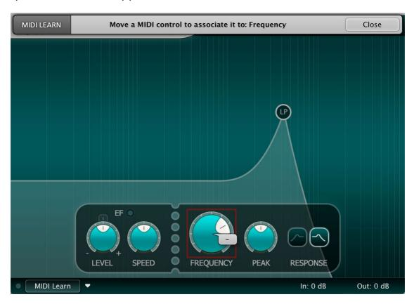
Click the **MIDI Learn** button in the bottom bar to enter MIDI Learn mode. The interface dims and the parameters that can be controlled are highlighted. Each parameter has a small text balloon that displays the associated controller number. Now do the following to associate a controller number with a parameter:
