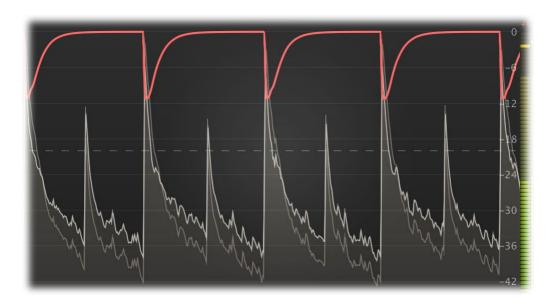
The top part of Pro-C 2 is actually a large animated level display, with the main compression controls panel floating above it. The level display visualizes the input and output level, together with the applied gain change. The input is shown in dark grey, whil the output is light grey with a light stroke, which makes it easy to see the exact effects of the applied gain reduction. The gain reduction itself is shown as a red line.
