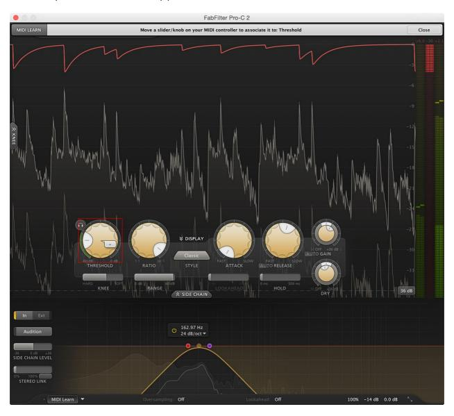
Click the **MIDI Learn** button in the bottom bar to enter MIDI Learn mode. The interface dims and the parameters that can be controlled are highlighted. Each parameter has a small text balloon that displays the associated controller number. Now do the following to associate a controller number with a parameter:
