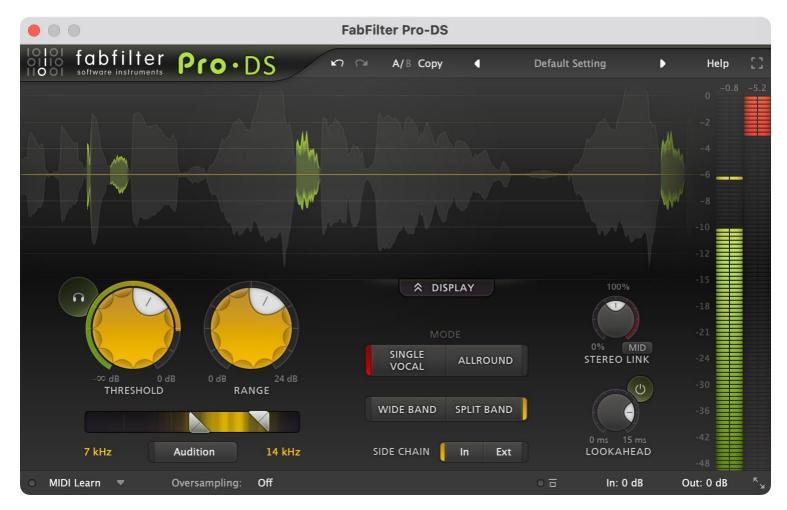
Key features include highly intelligent 'Single Vocal' detection to detect sibilance in vocals, transparent program-dependent compression/limiting, high-quality 64-bit internal processing, adjustable threshold, range and detection HP and LP filtering, Wide Band or linear-phase Split Band processing, optional look-ahead time up to 15 ms, adjustable stereo linking with optional mid-only or side-only processing and up to four times linear-phase oversampling.
