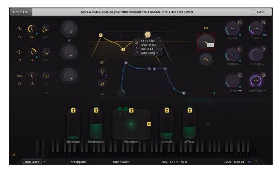
Click the **MIDI Learn** button in the bottom bar to enter MIDI Learn mode. The interface dims and the parameters that can be controlled are highlighted. Each parameter has a small text balloon that displays the associated controller number. Now do the following to associate a controller number with a parameter:
