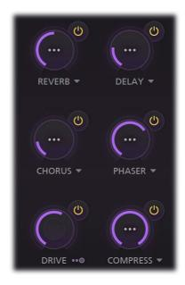
For each effect, you'll see a large **Amount knob**, and an **Enable/Disable button**. The menu button ▼ to the right of an effect label gives access to **presets per effect**. Clicking in the center of the knobs will open a panel with options per effect. While dragging to create modulation connections, you can hover above the knobs to open the panels.
