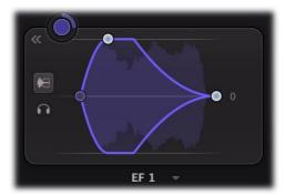
In the graphical **envelope controller** you can click and drag the dots to customize the attack and release times of the EF, which controls how the signal is smoothed.
