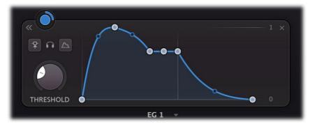
The expanded interface contains a large graphical envelope controller with triggering controls on the left.
