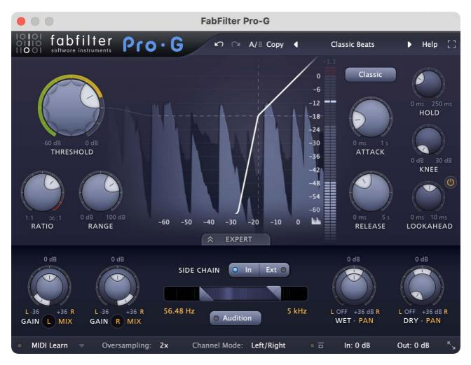
Key features include five meticulously tuned, program-dependent expander/gate algorithms, including an Upward expansion style, high-quality 64-bit internal processing, adjustable threshold, ratio and range, attack and release settings, adjustable hold time up to 250 ms, optional look-ahead time up to 10 ms, mid/side processing, up to four times linear-phase oversampling and an expert mode that offers highly customizable side chain options.
