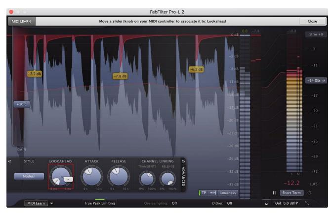
Click the **MIDI Learn** button in the bottom bar to enter MIDI Learn mode. The interface dims and the parameters that can be controlled are highlighted. Each parameter has a small text balloon that displays the associated controller number. Now do the following to associate a controller number with a parameter:
