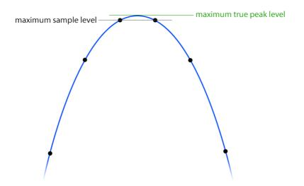
As illustrated by this image, the analog signal (blue) has a peak (green) that is higher than the sample peaks in the digital signal. Peaks like these are called inter-sample peaks or **true peaks**. Today, many commonly used metering/loudness standards, like <u>EBU R128 or ATSC A/85</u> impose a maximum allowed true peak level.
