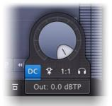
The **Output Level** knob plays an important role: it sets the desired maximum output level for the limiter. It seems natural to set it to 0.0 dB: you want the output to be as loud as possible, right? Not so fast.
