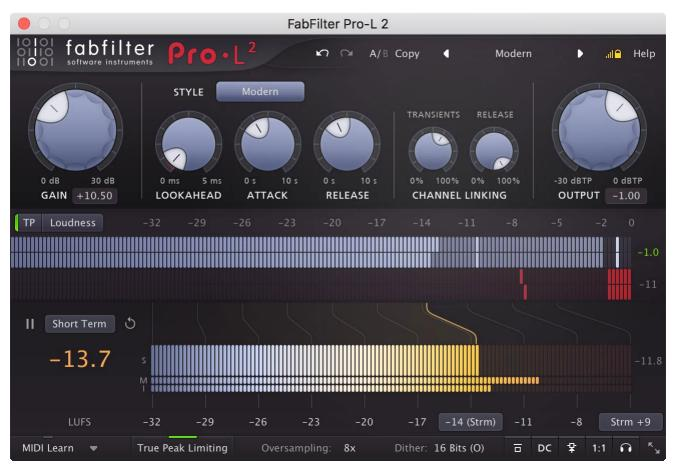
In Compact view, you can adjust the gain and the output level also by clicking and dragging on the level readouts below the Gain and Output knobs. Like with any knob, double-click here to type a value directly.
