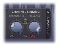
In the **first half of the range** (from "0% Stereo" to "100% Stereo"), the Transient and Release link knobs work the same as in the stereo version of the plug-in: it controls the amount of linking between L and R channels (e.g. L/R, Ls/Rs, Lc/Rc or Lts/Rts). However, every stereo pair's linking is still independent of the other stereo pairs.
